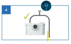
If the discharge takes place in a direct downwards way, provide for an aerator valve placed at the highest point to avoid the siphoning phenomenon.
