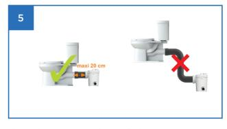
The appliance must not be installed **more** than 20 cm behind the toilet, nor at a lower level than the bowl.
