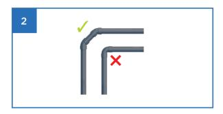
For the installation of connection elbows on the drainage piping, use 2 x 45° elbows rather than one 90° elbow.
