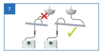
No sanitary appliance must be connected to the small diameter drainage pipe **specific to the macerator.**
