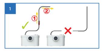
Vertical pumping must take place at the start of the DISCHARGE (1). From the highest point of the discharge (2), an incline of at least 1% is necessary.
