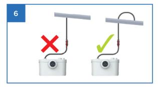
The macerator discharge pipe must be connected to the downspout from above, following the direction of flow.
